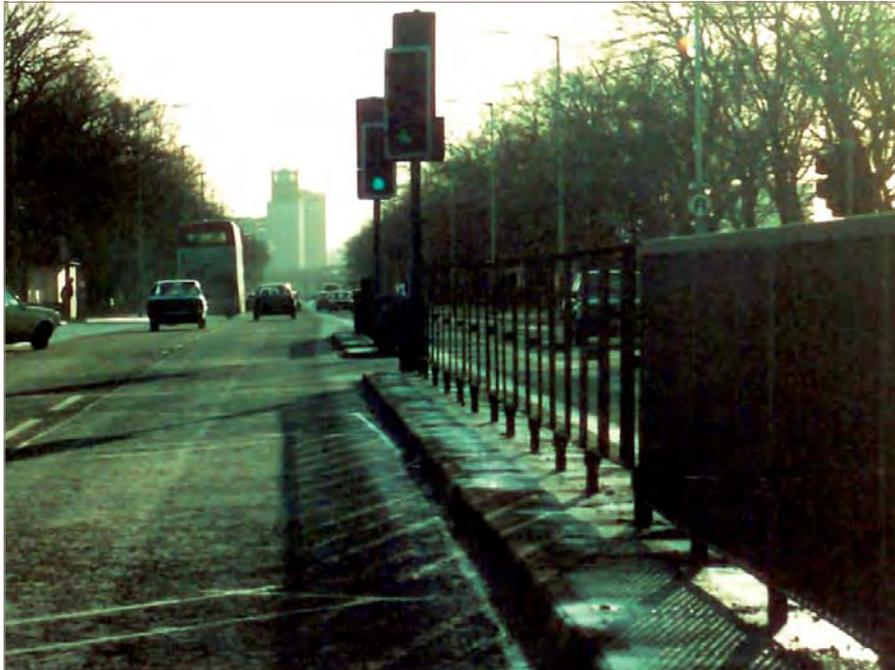
Fig. 2. Guardrail replacement by Visirail restored visibility for right-turning vehicles at this junction, leading to an 80% saving in accidents.
